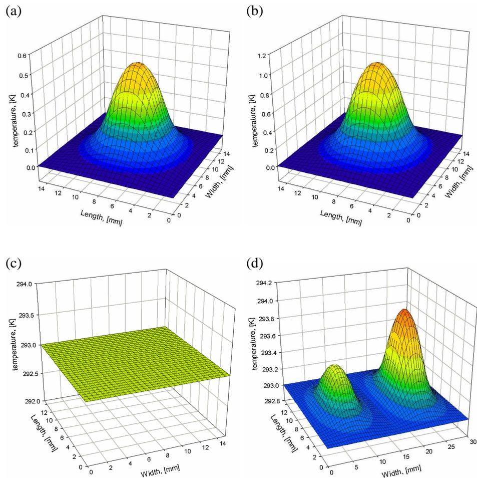
Fig. 5. Temperature distributions: (a) obtained by (4) with the lighting source parameter of 6.46 K/s, (b) also by (4) with the lighting source parameter of 12.92 K/s, (c)  $u_0$  – constant room temperature, (d) after summing up (a), (b) and (c) solutions.
