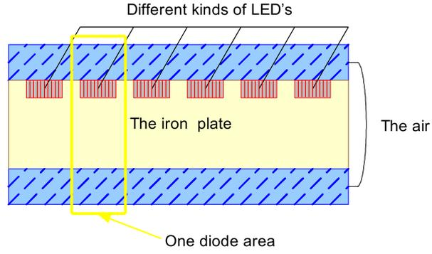
Fig. 3. The separation of the system (one LED system).
